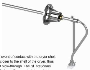
The special pick-up shoe has a PTFE sole to prevent damage in the unlikely event of contact with the dryer shell. The rigid mounting and protective PTFE sole enable positioning of the shoe closer to the shell of the dryer, thus ensuring effective condensate removal with minimal differential pressure and blow-through. The SL stationary siphon is recommended for use in open gear machines with the Deublin H Series self-supported steam joint.
