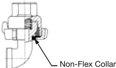
The non-flex collar design is used to prevent side flexibility. This swivel is used at the top anchor point to prevent lateral movement of long pipes. Only one non-flex collar swivel is to be used per dog-leg, otherwise binding of the assembly will occur.
