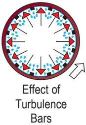
**Deublin** carbon steel bars also match the thermal expansion characteristics of the dryer vessel, to eliminate failures due to buckling, fretting and excessive wear. Stainless steel turbulence bars are recommended for cooling and swing cylinder applications.
