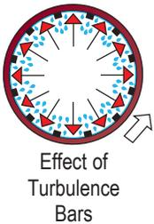
**Deublin** carbon steel bars also match the thermal expansion characteristics of the dryer vessel, to eliminate failures due to buckling, fretting and excessive wear. Stainless steel turbulence bars are recommended for cooling and swing cylinder applications.
