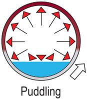
Condensate in full cascade provides the most efficient heat transfer. However, as machine operating speeds increase beyond approximately 305 MPM (1000 FPM), for 1.5 meter (5 feet) diameter dryer, centrifugal force causes the condensate to cling evenly around the shell of the dryer, a condition known as “rimming.” When this occurs, heat transfer efficiency deteriorates.
