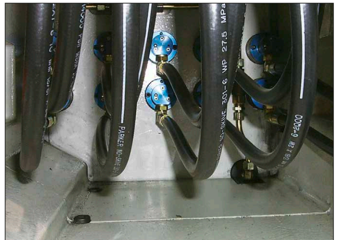
Deublin 1117 Bearingless Unions on Automotive Transfer Line.
